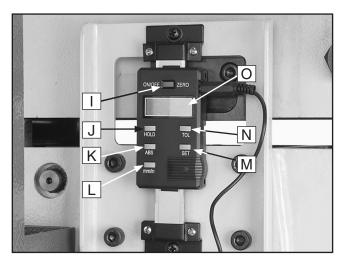
**Figure 3**. Infeed table digital sensor and controls.
